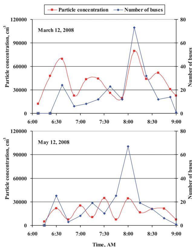
**Fig. 2** Comparison of the particle number concentration ( $d_p \geq 20\text{ nm}$ ) measured in 15 min intervals using a P-Trak with the number of school buses arriving and departing from the test site during one period in March and May.
