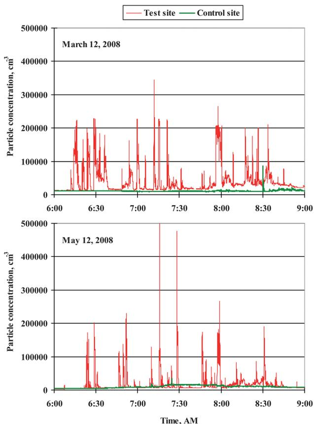
**Fig. 1** Comparison of the particle number concentration ( $d_p \geq 20$  nm) measured in 1 s intervals using a P-Trak for one period in March and May at the test and control sites.
